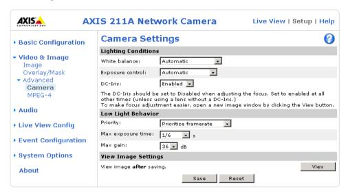
To compensate for the lighting conditions, the white balance and exposure control can be adjusted. If available, DC-Iris should always be enabled except during focusing, or when using a non-DC-Iris lens.
